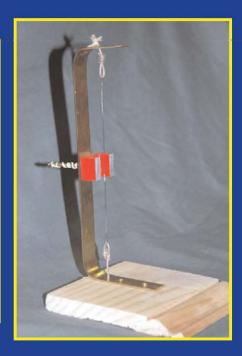
Connect two wire leads from the battery terminals. Alligator clips are helpful for securing the opposite ends of the leads to the flexible wire. (Be sure to strip or sand the insulation from the flexible wire to insure good contacts.) A switch in the circuit can aid in your presentation. Observe the flexible wire move when the current is applied. The movement may be determined by the size, strength and exact shape of the horseshoe magnet.
