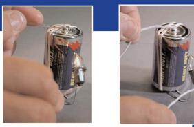
Now try the experiment with a rubber band and string. The bulb will not come on. This is because r ibber and cotton fibers are **insulators**. They will not allow electricity to pass, and thus, will not c implete the electrical circuit. Now repeat this experiment with other objects. Can you classify these materials as conductors or insulators?
