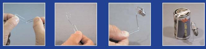
1.) Bend the paper clip at a right angle. 2.) Bend a small loop in one end of the paper clip [Hint: a fat pencil helps] 3. Angle the loop backwards slightly and place the flashlight bulb inside the loop. 4. Double the heavy rubber band and secure the paper clip firmly to the bottom of the battery. [Hint: sanding the paper clip where it touches the battery and bulb helps make good electrical contacts.
