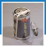
1.) Bend the paper clip at a right angle. 2.) Bend a small loop in one end of the paper clip [Hint: a fat pencil helps] 3. Angle the loop backwards slightly and place the flashlight bulb inside the loop. 4. Double the heavy rubber band and secure the paper clip firmly to the bottom of the battery. [Hint: sanding the paper clip where it touches the battery and bulb helps make good electrical contacts.
